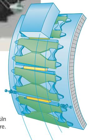
Splined kiln tyre fixture.
