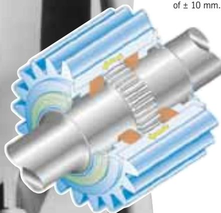
The use of a self-aligning pinion ensures that an optimum contact pattern is achieved over the entire width of the tooth gearing. The self-aligning pinion compensates any thermal distortion of the kiln shell and associated wobbling of the girth gear. In comparison to the rigid drive mechanism, the dimensions of girth gear and pinion are about 20 % smaller, due to the improved tooth
