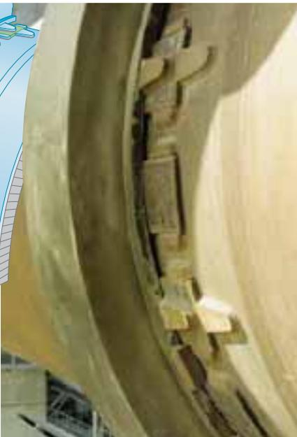
bearing pattern and the full frictional connection. This back gear unit is also a favourably priced refurbishment measure for existing kilns.
