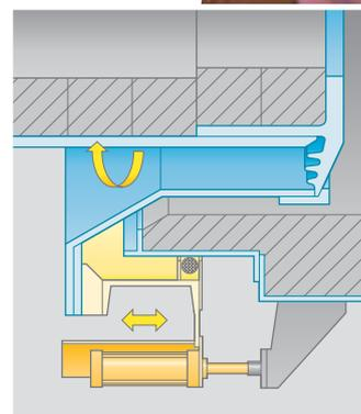
Pneumatic rotary kiln outlet seal.
