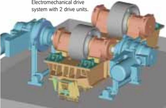
In order to prevent contact surface wear during operation of the POLRO®, the axes of rotation of supporting rollers and kiln tyres are always parallel. This is ensured by a positioner, which adjusts the rollers relative to the tyre during the kiln operation.
