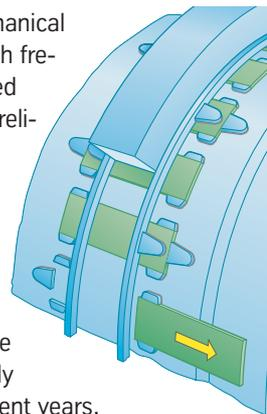
Self-aligning drive pinion: the design permits a tilting of  $\pm 10$  mm.
