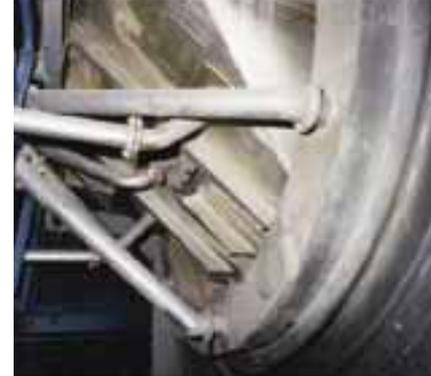
Because Polysius rotary kiln seals are highly efficient, robust and wear resistant they save energy and are extremely durable.
