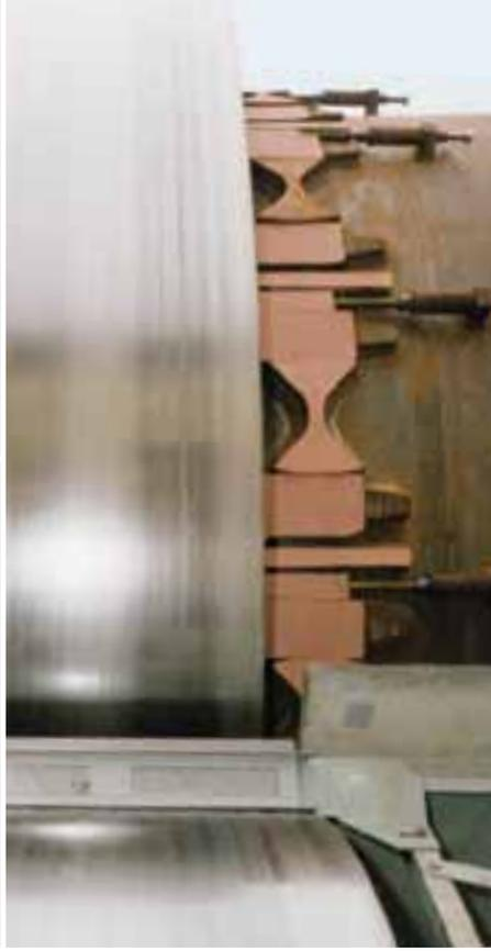
Splined kiln tyre fixture.
