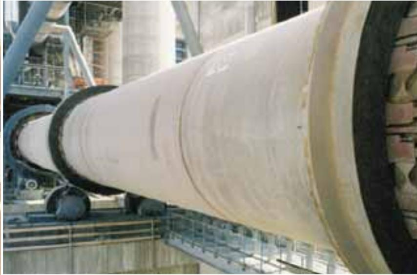
Rotary kiln supported on 3 roller stations.
